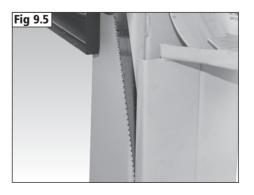
Fit the new blade to the bandsaw, ensuring the teeth of the blade point downwards and towards the front of the machine, **Fig 9.6**.
