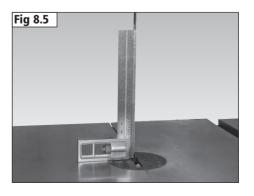
Once the table is at 90° to the blade with a square, the angle scale pointer can now be adjusted to point to 0° as shown in **Fig 8.6** using a Phillips screwdriver.
