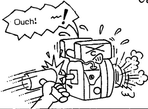
When the pulley is tapped lightly to the shaft by a plastic hammer, it should fit properly to the shaft.
