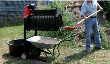
Thanks to the sieve drum design, nothing is in the way when feeding it.
