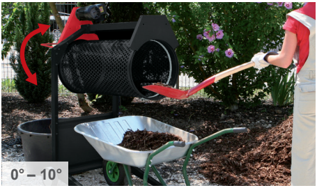
By selecting the drum angle, you can control the speed of the material passing through.
