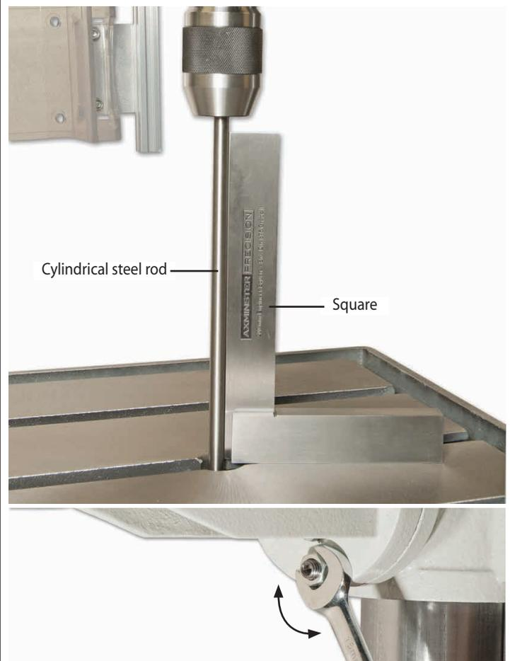
1. The cast iron table can be tilted 45° degrees in both planes, to tilt the table you will need to first remove the tables 90° locking pin. To remove the locking pin use a 10mm spanner, turn the nut clockwise to draw the pin out. Remove the pin and place safely aside, see fig 48-49. Loosen the tilt clamping bolt and tilt the table to the desired angle then retighten the bolt.
