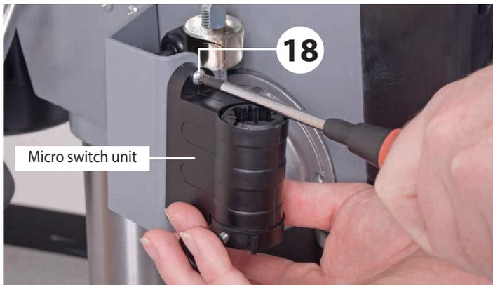
7. Undo the clamping knob to the side of the micro switch sufficiently to allow the guard rail to slide up through the centre of switch.
