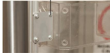
9. Introduce the chuck guard rail (7) up through the centre of the micro switch and nip up the clamping knob to lock the chuck guard in place, see fig 35.
