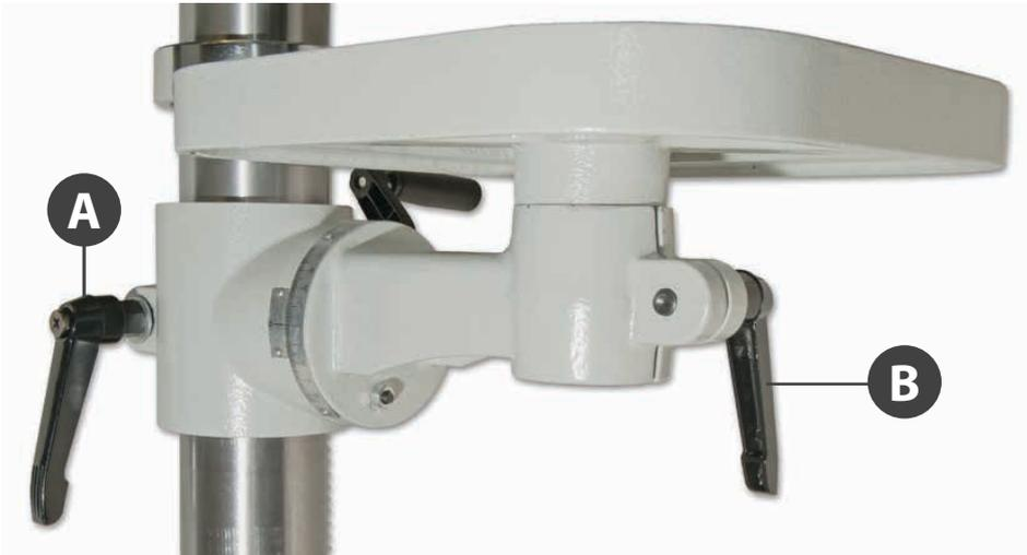
Lift and shift handle (A) for securing the table mounting arm
