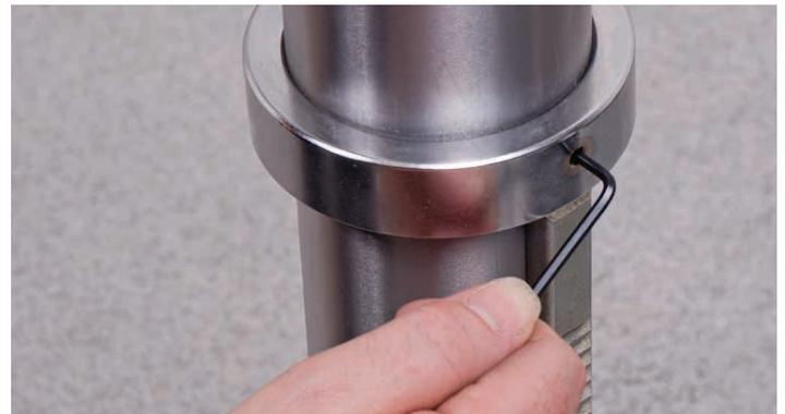
5. Locate and fit the crank handle (10) to the shaft, ensuring that you tighten the grub screw onto the machined flat on the shaft, this will keep the worm gear in position, see fig 10-11.
