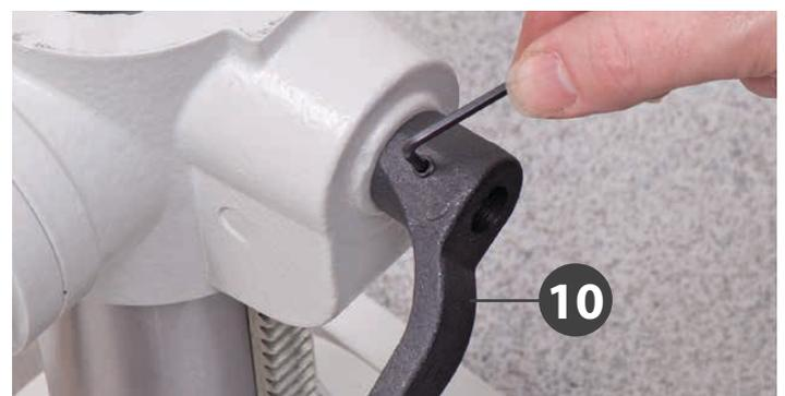
6. Check that the mounting bracket can be driven up and down the column and can swivel around the pillar. Locate the lift and shift handle (8) and screw it into the threaded hole to the rear of the mounting bracket arm and tighten, see fig 12. **DO NOT OVERTIGHTEN as the cast iron arm could break.** Check it has 'pinched' up on the column and the bracket is immobile; both in its up and down travel and swivel movement.
