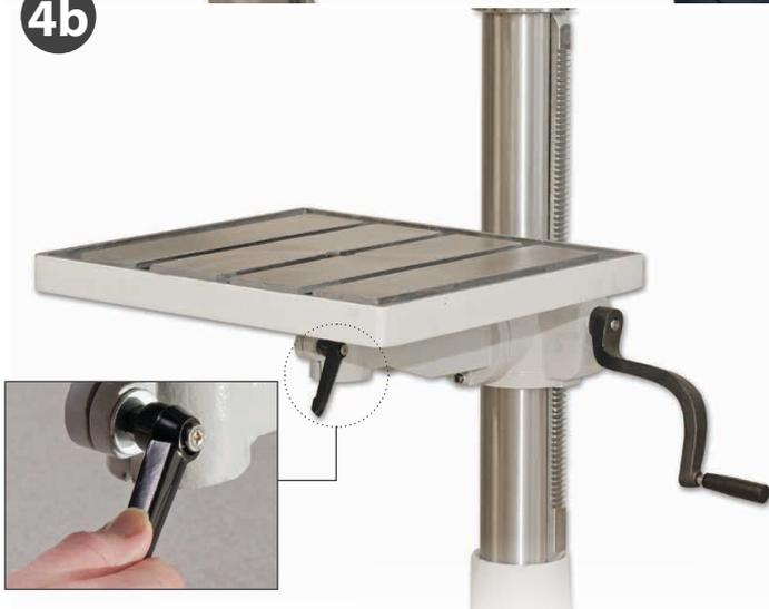
7. Screw in the remaining lift and shift handle (8) into the threaded hole to the end of the mounting arm. **DO NOT OVERTIGHTEN as the cast iron arm could break.** Lower the drill table (4,4a,4b) spigot into the machined hole to the front of the mounting arm and tighten the handle until it has 'pinched' up on the drill table's spigot and the table is immobile, see fig 13-14-15.
