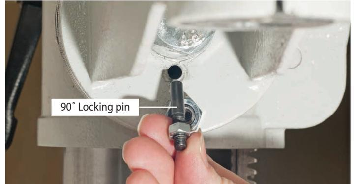
2. To set the table back to 90° degrees, loosen the clamping bolt, position the table back in the horizontal plain and insert the locking pin into the machined hole in the support arm. Adjust the nut so it protects the end of the threaded pin and using a high faced mallet tap the locking pin into place.
