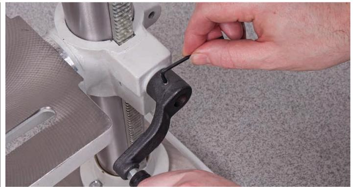
6. Check that the bracket can be driven up and down the column and can swivel around the pillar. Locate the lift and shift clamping handle (10) and screw it into the threaded hole to the rear of the mounting bracket arm (2) and tighten, see fig 11. Check it has 'pinched' up on the column and the bracket is immobile; both in its up and down travel and swivel movement.
