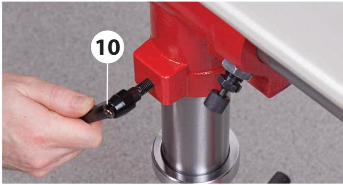
3. Locate another lift and shift handle (10) and screw it into the threaded hole for the Horizontal clamp assembly, see fig 22.
