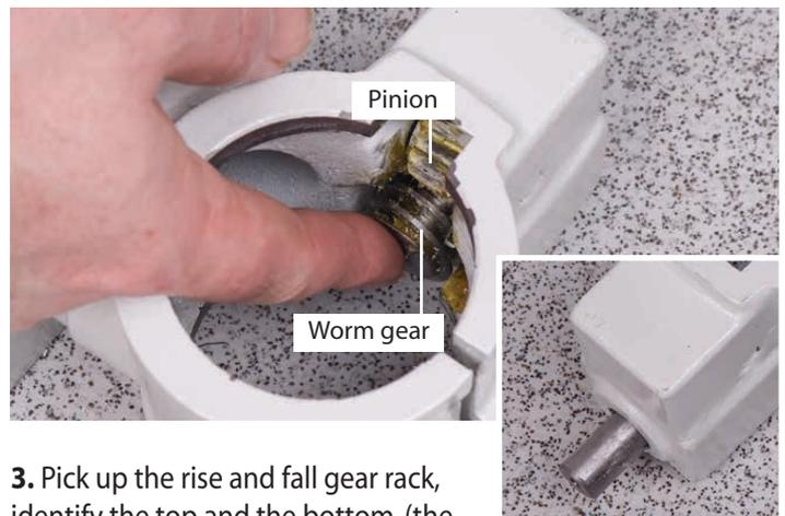
3. Pick up the rise and fall gear rack, identify the top and the bottom, (the rack gearing is cut asymmetrically, with the gear cut extending closer to the bottom), make sure you have the rack the right way up, as it will allow you to drive the drill table up and down over its full range, see fig 5.
