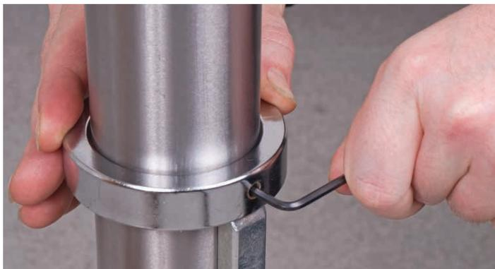
5. Locate and fit the crank handle (9) to the shaft, ensuring that you tighten the grub screw onto the machined flat on the shaft, this will keep the worm gear in position, see figs 9-10.
