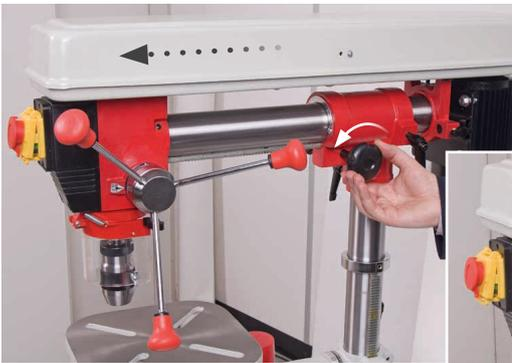
Turn the horizontal adjusting knob anti-clockwise to move the column forward
