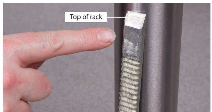
4. Fit the rise and fall rack into the square recess in the mounting body casting, ensure that it is engaged with the pinion, see figs 6 and lower the combined mechanism over the column (1). Allow it to slide down the column until the rise and fall rack is located in the cup chamfer in the top of the mounting flange, see figs 7. Replace the cup chamfered retaining
