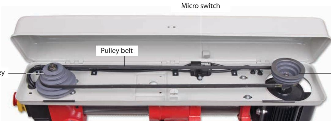
Quill pulley      Pulley belt      Micro switch      Motor pulley
